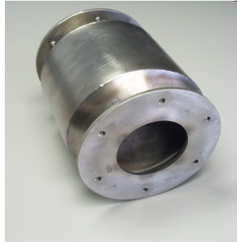
Canned DOC with flanges designed for the Mercedes Benz OM904 4 cylinder engine
