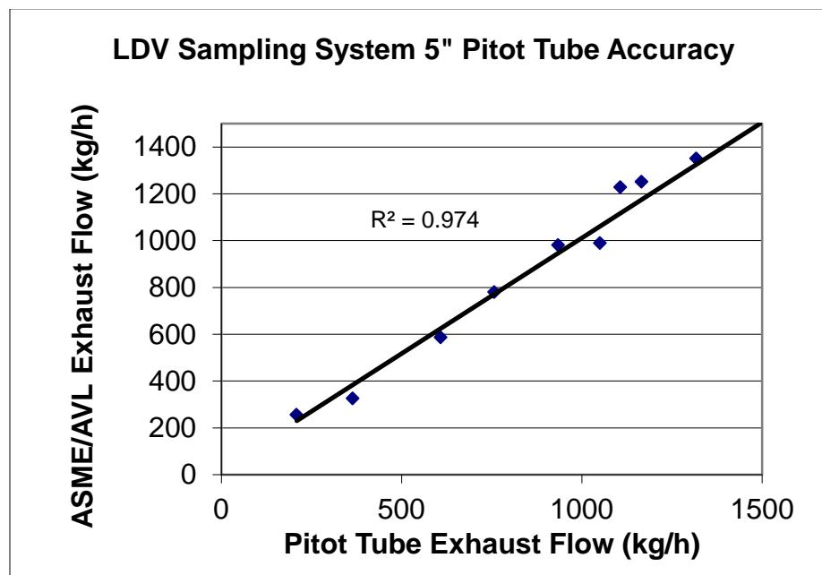
**Figure 7** - Pitot tube calibration chart
