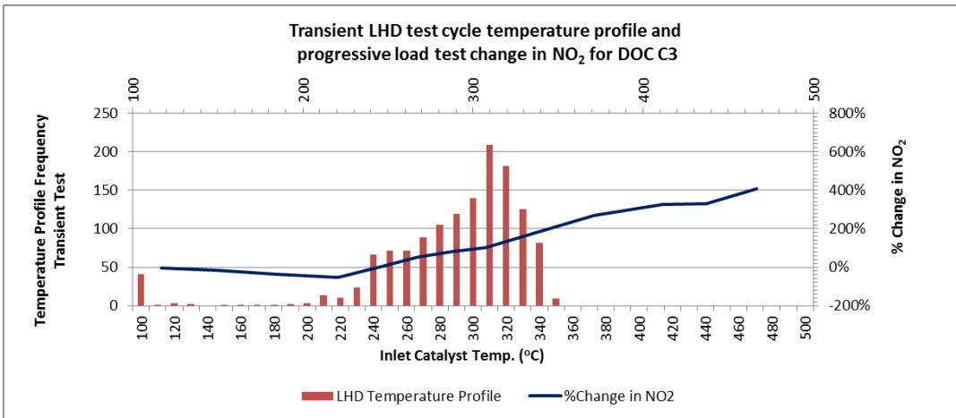
**Figure 12** - Transient mine LHD test cycle temperature profile and progressive load test NO<sub>2</sub> percent change for DOC C3
