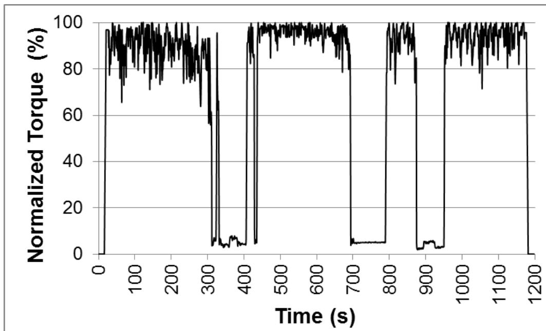
**Figure 2b** - Normalized torque over utility vehicle cycle
