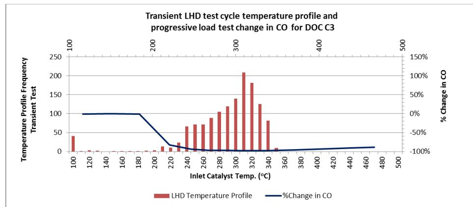
**Figure 10 - Transient LHD test cycle temperature profile and progressive load test CO percent reduction for DOC C3**
