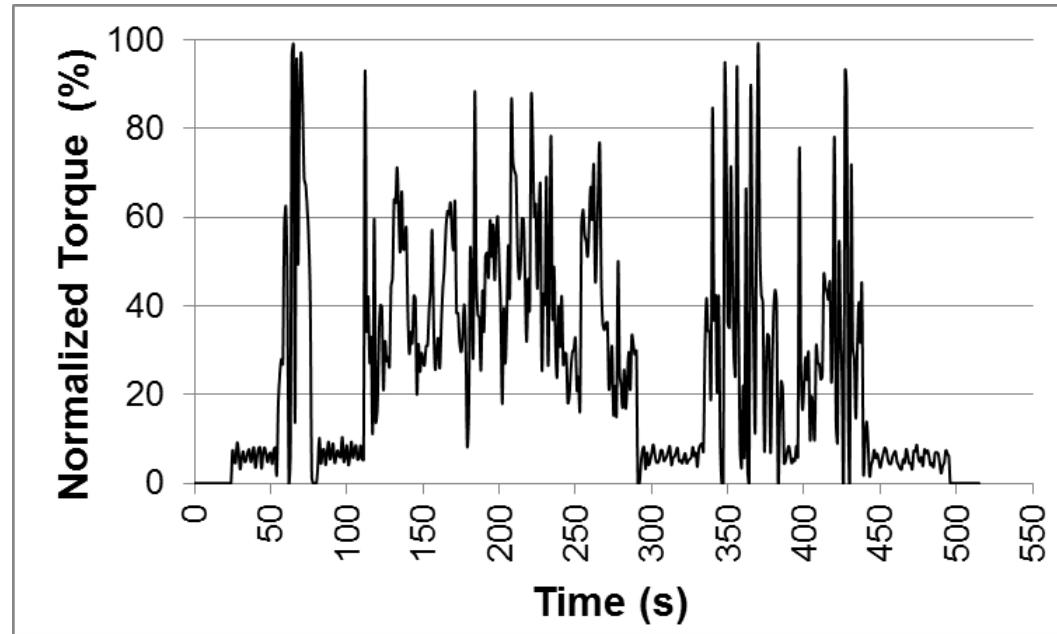
**Figure 4b** - Normalized torque over tractor vehicle cycle
