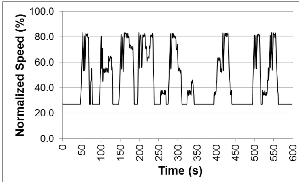
**Figure 3a** - Normalized speed over pickup vehicle cycle
