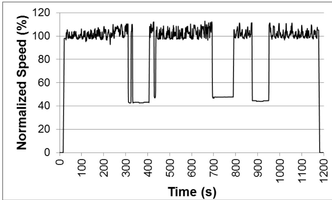
**Figure 2a** - Normalized speed over utility vehicle cycle
