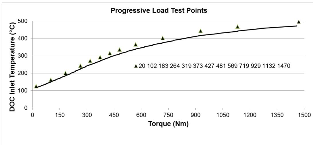
**Figure 9 – Exhaust temperatures with engine torque over progressive load testing**
