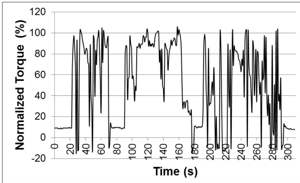
**Figure 1b** - Normalized torque over LHD vehicle cycle
