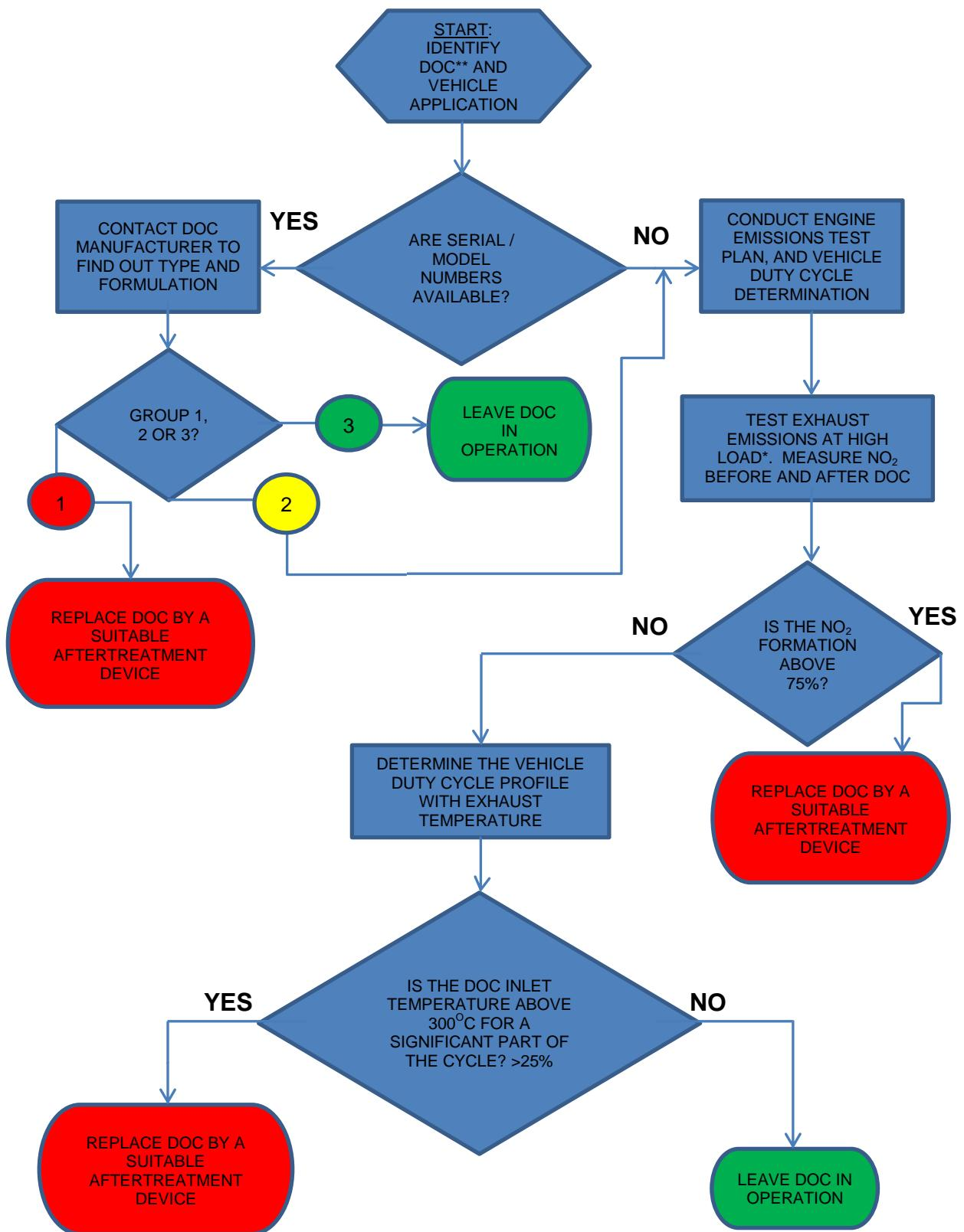
\* The engine emissions test must be performed at high load to ensure the DOC is in its normal operating temperature range. The transmission stall or hydraulic stall tests as mandated by the Ontario MOL are acceptable.
