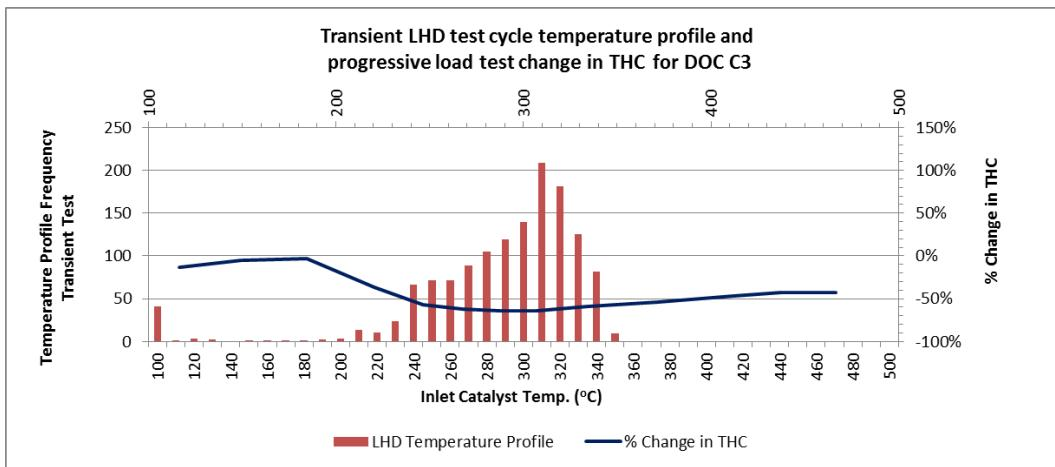
**Figure 11 - Transient LHD test cycle temperature profile and progressive load test THC percent reduction for DOC C3**
