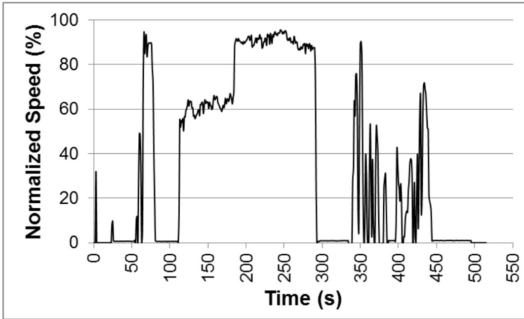
**Figure 4a** - Normalized speed over tractor vehicle cycle
