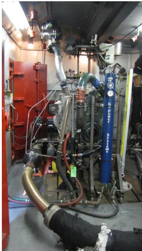
**Figure 8 –** DOC installed in the total exhaust system
