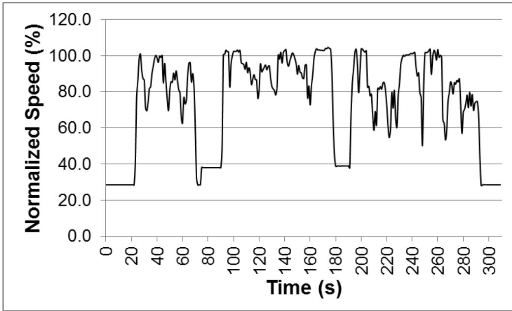
**Figure 1a** - Normalized speed over LHD vehicle cycle
