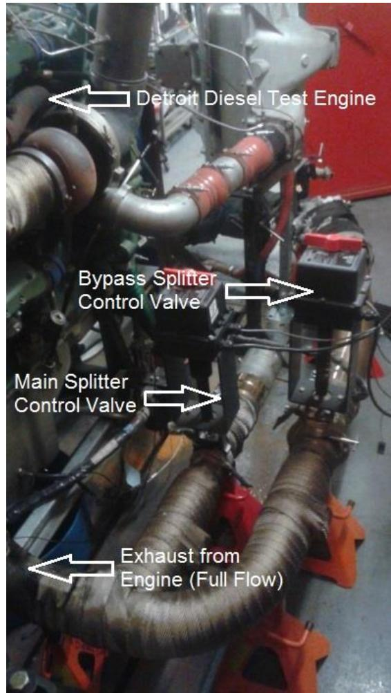
**Figure 5 - Exhaust flow splitter rig**
