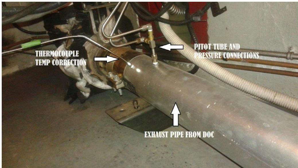
**Figure 6** - Exhaust flow measuring pitot tube and thermocouple
