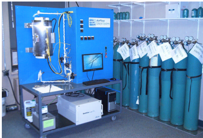
Figure 1: Synthetic Gas Reactor Set Up
